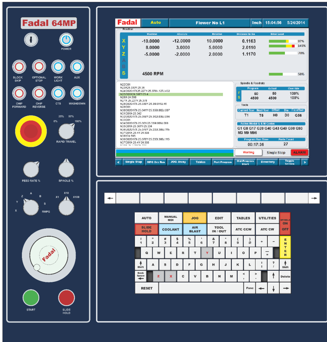
Figure 1-1 Physical Layout of Fadal 64 MP
